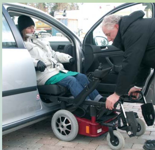
Release the chair's wheel unit from the swivel base.
