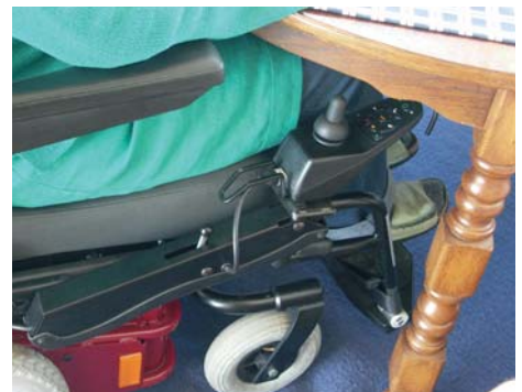
The arm of the control box can be lowered – an advantage when sitting at a table, for instance.
