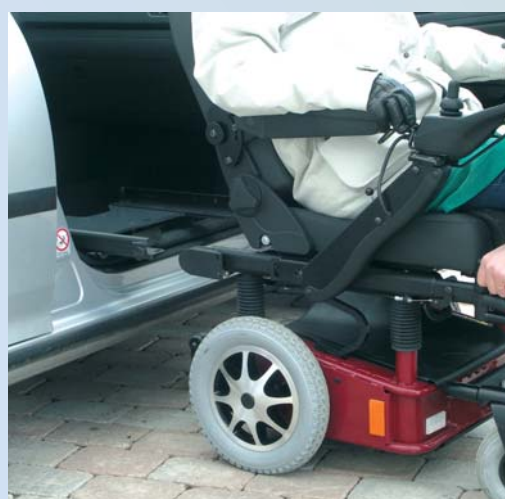
Disconnect the motors so the wheelchair can be rolled manually. Dock the chair to the rails on the swivel base.
