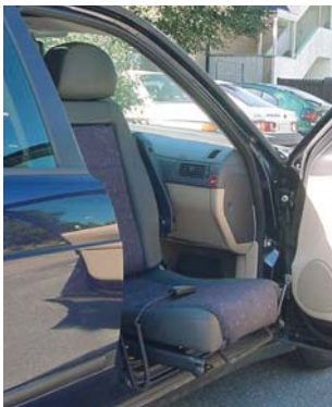
The Turnout swivel base turns the chair outwards, so Carony Go can be docked to the car.
