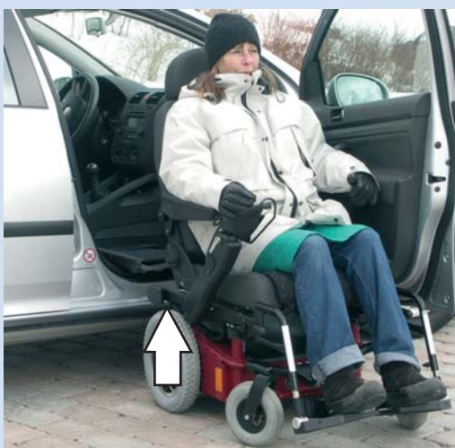
Using the control box, raise the wheelchair to the same level as the swivel base.
