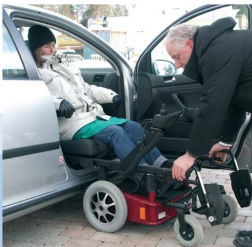
Release the chair's wheel unit from the swivel base.
