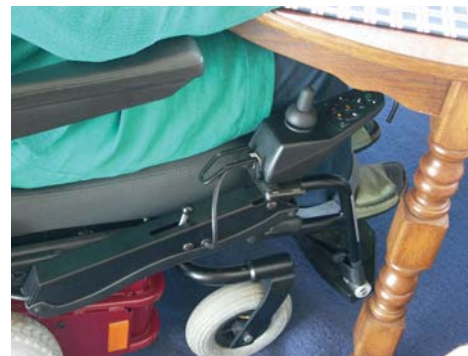
The arm of the control box can be lowered – an advantage when sitting at a table, for instance.
