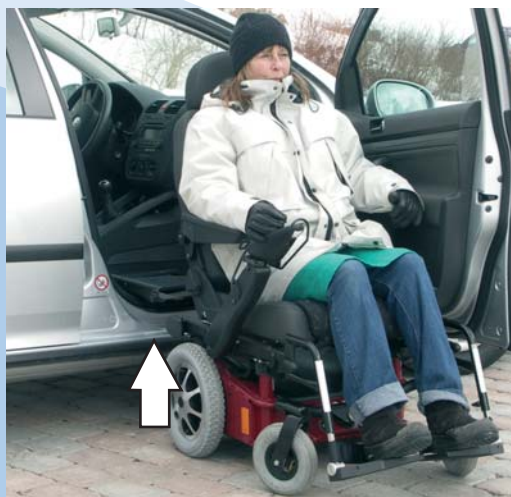
Using the control box, raise the wheelchair to the same level as the swivel base.
