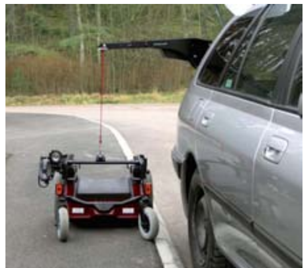
Carolift 6000 /6900 can pick up a wheelchair from the side of the vehicle.
