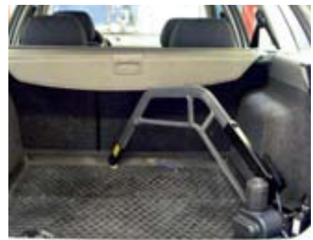
The hoist folded to the floor
